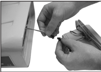
Figure 6. Unplugging the battery.
